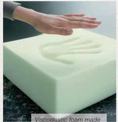
*Viscoelastic foam made from BASF products is thermosensitive. It adjusts to the shape of the body by reacting to body heat and pressure. Foam follows function.*
