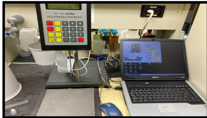
Figure 1 – Benchtop Rheometer Set-Up
