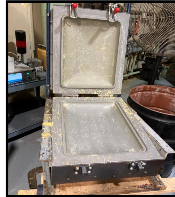
Figure 2 – Pillow Mold Set-Up
