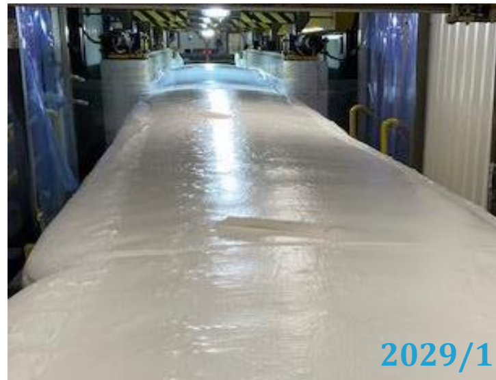
Figure 4 – Handling of Foam Buns on Pilot Scale Slab Machine
