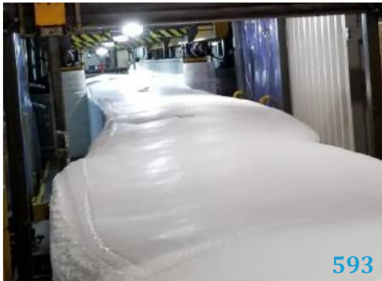
Figure 4 – Handling of Foam Buns on Pilot Scale Slab Machine
